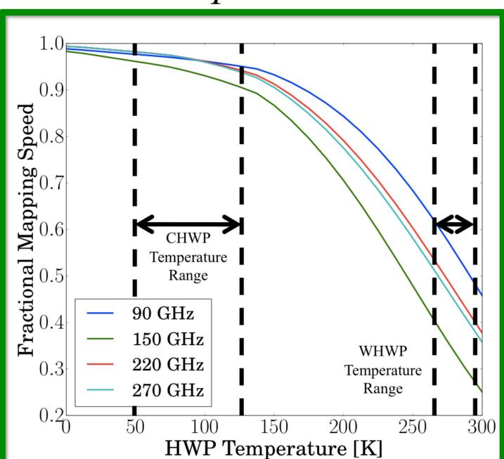
• The CHWP target temperature range is 50 - 125 K where its impact on PB2 mapping speed is < 10%
