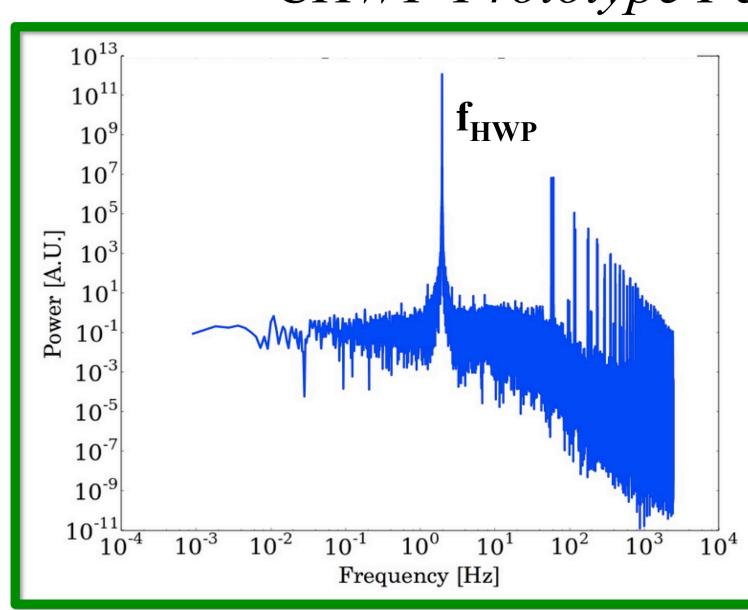
The prototype rotational power spectrum shows good encoder signal-to-noise, rotational stability, and lowfrequency performance, validating the magnetic motor + bearing design
