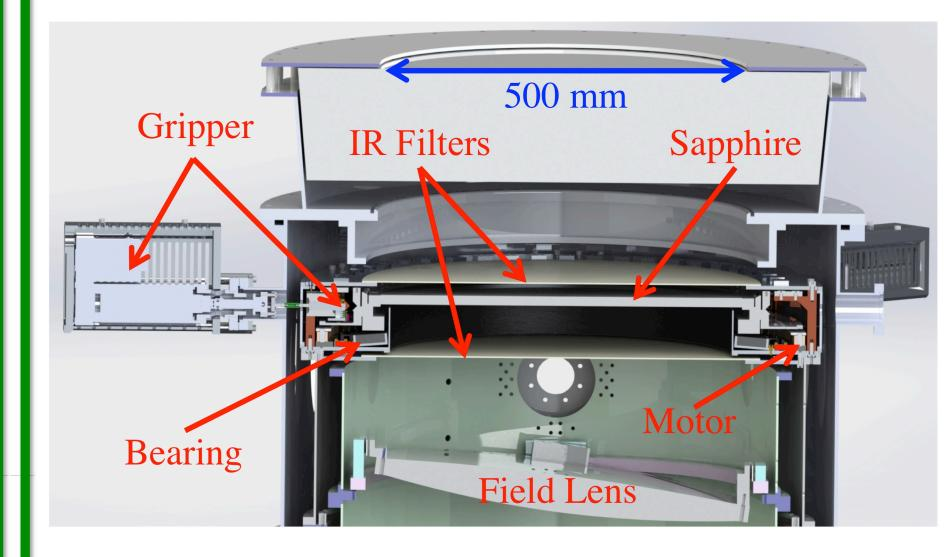
A full-scale CHWP will be deployed on PB2b in 2018 and is under evaluation in a test cryostat at LBNL
