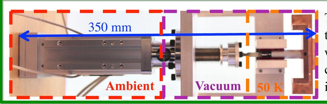
Three gripper arms hold the CHWP rotor when warm, cool it via conduction, and release it when cold
