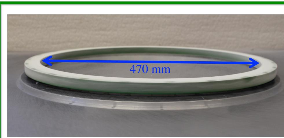
A superconducting magnetic levitating thin-section bearing from ATZ GmbH operates with a friction coefficient  $\mu_k < 10^{-7}$  at 77 K and dissipates < 10 mW at 2 Hz rotation
